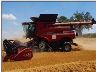
Case IH Axial Flow 8240 (Ex-Demo) - 35ft, side knives, full guidance, suspended tracks, Xtra Chop. £ POA
