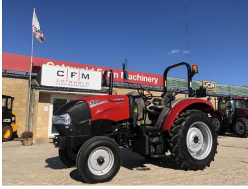
Case IH 55A - 2WD, 8x8 manual gearbox with mech shuttle, 2 mech spool valves, ROPS.
