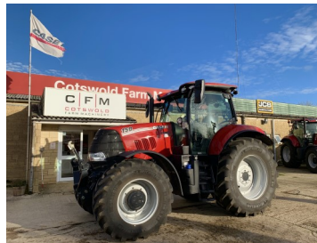
Case IH Puma 150 Xtra - 50kph, semi-powershift, full suspension, front links, 4 mech spools, 3 speed
