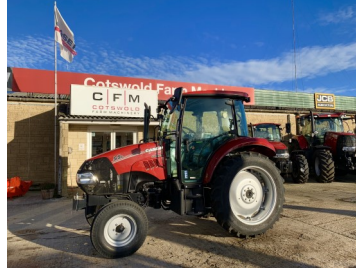
Case IH 55C - 2WD, 12x12 manual gearbox with power shuttle, 1 mech spool valve, pickup hitch.
