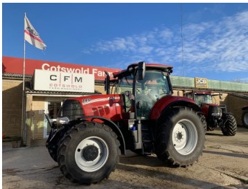
Case IH Puma 140 X - 50kph, semi-powershift, full suspension, front links, 4 mech spools, 3 speed PTO.
