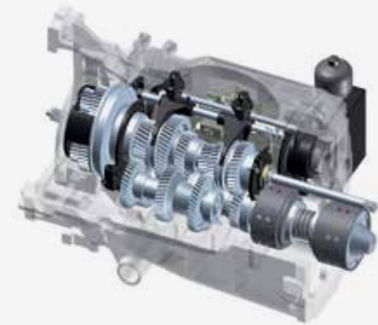
CVX transmission – stepless drive between 0-50 kph
