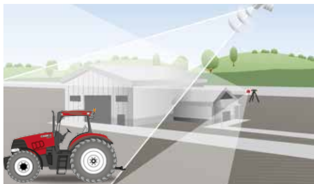
xFill bridges RTK signal gaps of up to 20 minutes.
