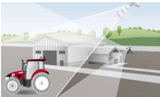
xFill bridges RTK signal gaps up to 20 minutes.
