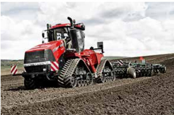
Magnum Rowtrac follows the same concept as Quadtrac with four points of contact to the ground.
