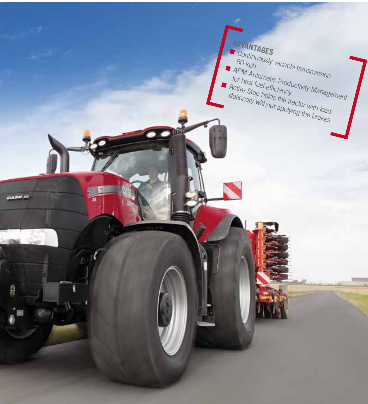
CVX transmission – stepless drive between 0-50 kph
