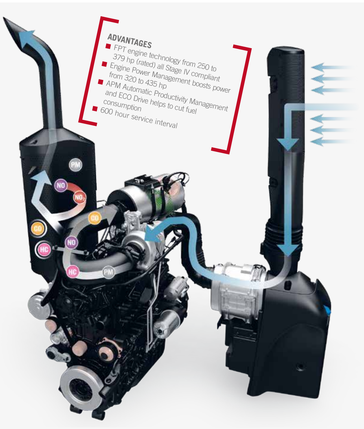
Perfect integration of engine and transmission – FPT Industrial in house engines.
