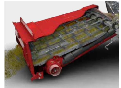
High capacity feeder, swallowing dense crop from the widest headers in industry without chocking
