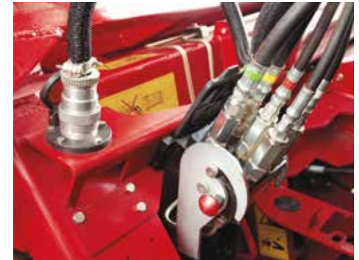
Mount the header in a matter of minutes with the single latch that connects all hydraulic services
