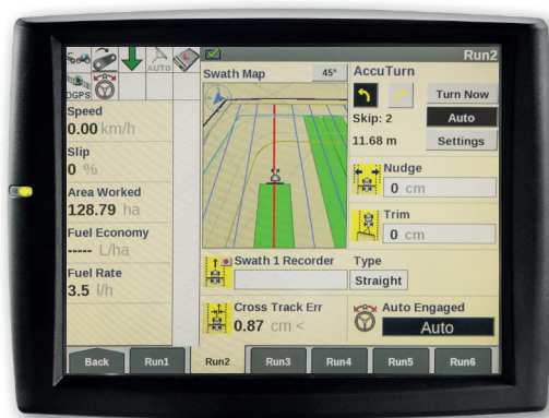
Automated turning process with AFS AccuTurn Pro
