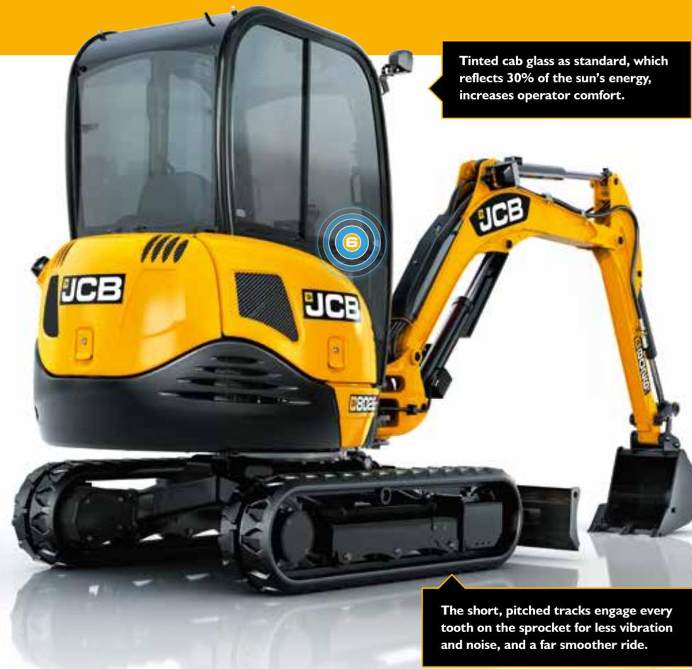
The short, pitched tracks engage every tooth on the sprocket for less vibration and noise, and a far smoother ride.
