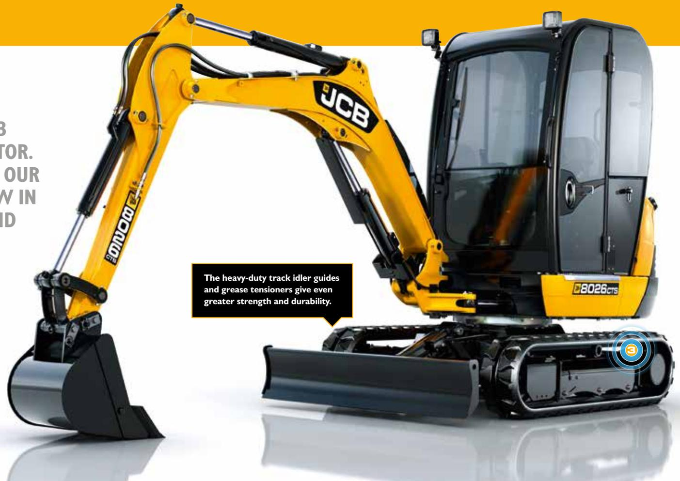
The heavy-duty track idler guides and grease tensioners give even greater strength and durability.
