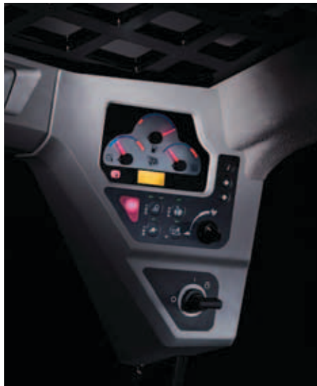
The right control panel features machine diagnostics, an electronic throttle and the skid steer's ignition.
