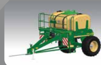
1 x 2,885 litres seed and 2 x 760 litres for total of 1,520 litres of liquid fertiliser.
