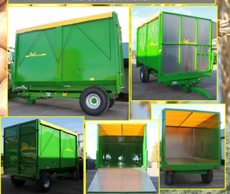
The AW Horse Muck Trailer is designed to be loaded by wheel-barrow or loader bucket. There is a spring assisted fold down ramp at the front and there are barn type doors at the rear. Fitted with hydraulic tipping and hydraulic brakes as standard. Optional extras available include fitted sheet, upgrade to  $400/60 \times 15.5$  tyres, full road lighting, removable sides.
