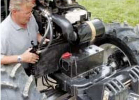
Filter can be removed without tools for quick maintenance.
