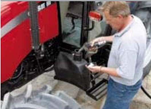
Refuelling at ground level with an easily accessible filler neck.
