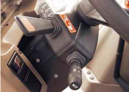
Two-speed Powershift transmission with thumb shift control.
