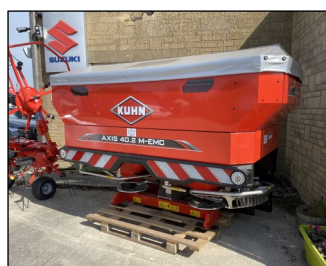
New Kuhn Axis 40.2 M-EMC VS8, 3200l hopper c/w cover, Quantron control, 18-28m discs, border control. £POA
