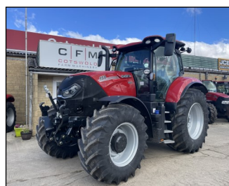
New Case IH Puma 150, 50kph semi-powershift, front sus, front linkage, 4 mech spools, LED worklights, external
