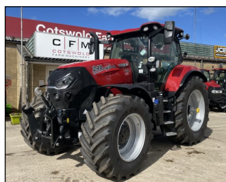
Demo Case IH Puma 240 CVX, 50kph, 4 elec spools, front links, accuguide complete, LED worklights. £POA
