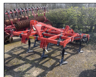
New Kuhn Cultimer L 300 T 3m mounted tine cultivator, traction bolt legs, 80mm shares & 350mm wings. £POA
