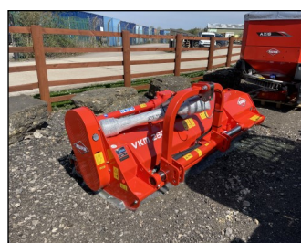
New VKM 280 rear mounted flail mower, 2.8m working width, hydraulic side shift, adjustable rear roller, 540/1000. £7,750
