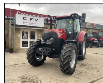
New Case IH Maxxum 125, 40kph, 16x16 semi-powershift, 3 mech spools, front & cab sus, LED Worklights. £POA
