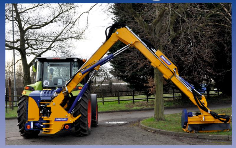
The Eagle flail mower is a 137 litre per min, 8.0m reach, non-parallel geometry, twin sided cutting straight arm machines with a telescopic outer arm and a hydraulic turntable for the attached implement. These durable professional contractor machines have a separate mainframe and oil tank and also a kingpost which allow's the arm set to be slewed through 180 degrees for twin cutting, left hand and right hand.
