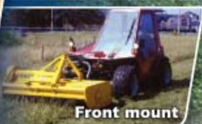
The Bandit trailed flail mower is aimed at professional users where efficiency and finish are a must. The Bomford Bandit mower range is built to withstand the toughest working conditions. Remaining manoeuvrable when mowing tight up to walls and obstructions. The flexible design of the Bandit allows it to be front or rear mounted simply by turning the A frame around (except B1200).
