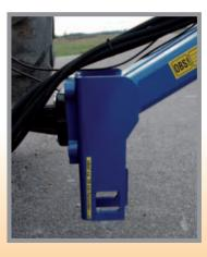
It is important to work with the correct drawing height app. 35 cm under the flange. (5.30-8.30)
