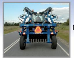
In transport position Maxiroll 2008 is only 2.50 m wide. The 8.30HD, 10.30 and 12.30 m versions are 3.00 m. All models are as standard equipped with road lights.
