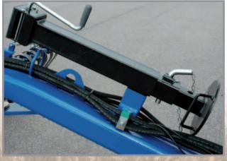
As standard the roller is equipped with jack, which during work has to be dismounted and placed in the holder on the drawbar.
