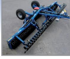
When the roller is open it can be lowered. The wheels will then smoothly come free of the ground. Now it is time to pressurize the outer sections. 33% weight on each section, put in floating position, the job can begin! (see picture below)
