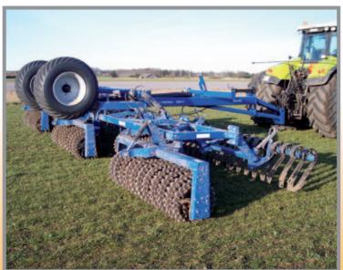
Maxiroll 10.30 and 12.30 consist of 5 sections, and like the other models in this range each section is equipped with hydraulic suspension and can follow the ground contours perfectly. Even with this wide working width optimum soil contact is achieved over the full working width. The 10.30m Maxiroll 2008 can be fitted with a hydraulic cracker board or harrow, and the 12.30m model has the hydraulic cracker board fitted as standard.
