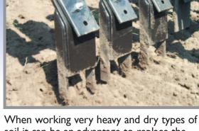
When working very heavy and dry types of soil it can be an advantage to replace the standard wearing parts by "crust crackers".
