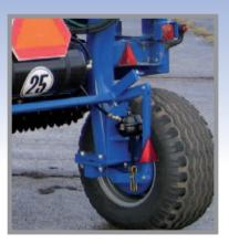
The rollers can be equipped with either hydraulic or air brakes. (Picture: air brakes)
