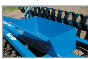
Stone trays can be added to each of the side gangs. The trays are emptied automatically when folding.
