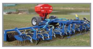
As an alternative to the crackerboard Maxiroll 2008 can be equipped with a 2 row harrow. The angle of the harrow can be adjusted by spindles and the adjustment of the depth is hydraulic.
