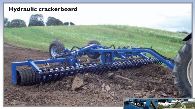
For seed bed preparation and levelling of the ground we recommend equipping the roller with a hydraulic Crackerboard. The improved ground clearance on Maxiroll 2008 facilitates an effective location for the Crackerboard providing optimum performance. The heavy duty spring steel tines have a greater vibration effect crushing clods and evening the surface. As standard the crackerboard is equipped with heavy 100x12 mm curved blades...
