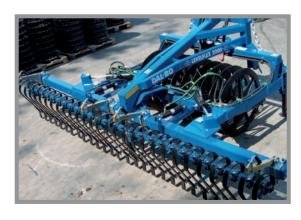
A 4.0 m hydraulic Crackerboard can be fitted to the special version of Levelflex 2008 1.5 m. The Crackerboard is hydraulically folded for transport; with a transport width is 2.5 m.
