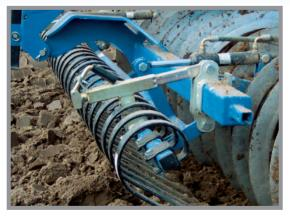
The working depth of the Crackerboard is hydraulically adjustable – even in work. This makes it possible to work to optimum effect in different soil types. The working angle is adjusted by spindles. Because of the special parallelogram suspension the working depth and the working angle are independently adjustable of each other. This makes it possible to work relatively aggressively providing a more intensive cultivation effect.
