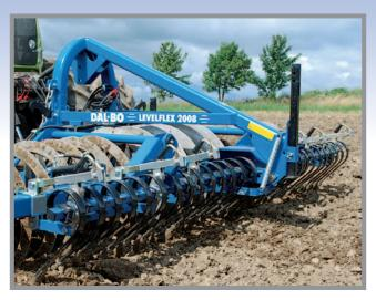
The front mounting and improved geometry pull the packer forwards, making it easier to control.
