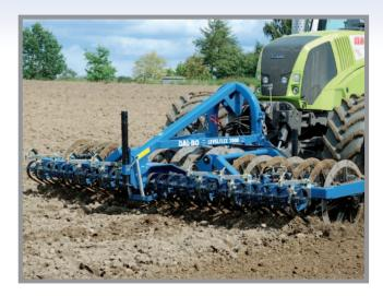
The flagships of the Levelflex 2008 range are the 4 & 6 m working width models. The hydraulic folding side sections give a transport width of only 2.9m. The hydraulic folding models are fitted with an automatic mechanical locking device for transport.
