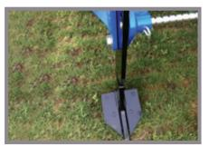
The working depth of the tines is adjusted via pin holes in the subsoiler leg. Hence, it is possible to work from 70 - 400 mm deep. Each tine has a shear bolt stone protection.
