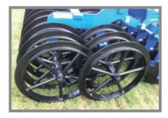
The standard double T profiled ring roller effectively crushes clods and consolidates the ground. The rings are self cleaning enabling the machine to work in very damp conditions.
