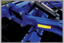
The working depth of the **SuperMax** is hydraulically controlled from the driver's seat. Two hydraulic rams simply adjust the pressure on the ring rollers, which carry the machine and ensure an even finish.
