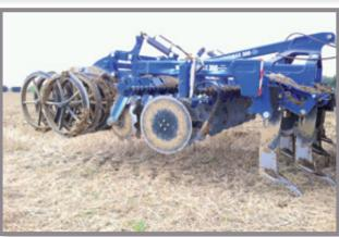
Heavy duty one pass cultivator 2.5 - 3 m working width
