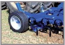
Support wheels are very effective for controlling the same working depth over the entire working width. They are standard on the 8.0 m and an option on the 6.0 m version.
