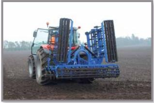
Heavy duty mounted seedbed cultivator Working width 5 – 6 – 8 m
