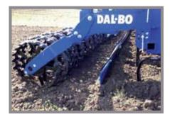
The standard cage roller can be replaced by a Crosskill roller. The 500/450 mm diameter has a unique capability of carrying the machine, even in very soft soil conditions. Made out of steel, the weight is limited, maintaining the superb cultivation effect of the Crosskill ring style. As an option levelling bar can be fitted in front of the roller.
