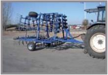
Despite its wide working width CultiTrail is only 2.5 m wide in Transport position. Folding and unfolding is controlled hydraulically from the tractor seat, which makes the job very easy for the operator.
