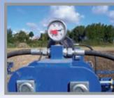
The semi-mounted **MaxiDiscs** are fitted with hydraulic weight distribution by using the well known Dal-Bo DUOFLEX system.This incorporates a hydraulic accumulator which ensures even weight distribution across the working width of the machine.
