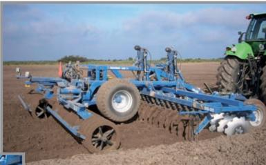
At the front the depth is controlled by the tractor linkage arms and support wheels at the outside of the disc sections. The support wheels ensure a uniform working depth – also in changing soil conditions.
