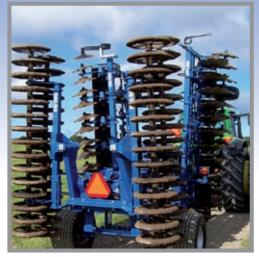
The semi-mounted models are under 3 m wide when in the transport position.
