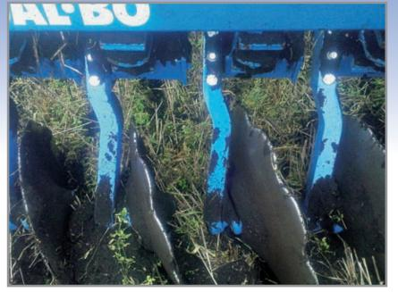
In the rubber system the 560x6 mm discs are fitted on individual hubs. The pre-tensioned system ensures a uniform working depth in all conditions.
