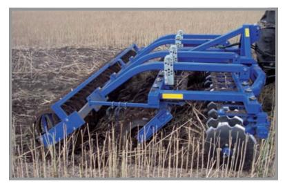
The semi-mounted **MaxiDiscs** are fitted with a HD 600 mm T-ring packer roller. The rings are made from 70x70x8 mm T-steel, facilitating a better carrying capacity and wear-ability. Furthermore the wider T-rings leave a finer soil structure.
