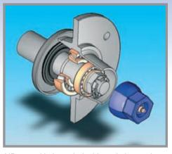
HD special hubs with double sealed conical roller bearings ensure a long life. The hubs must be greased every 50 hours.
