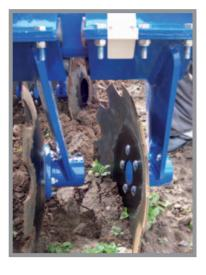
The angled 520 mm jagged discs have a superb mixing effect — also in difficult conditions.
