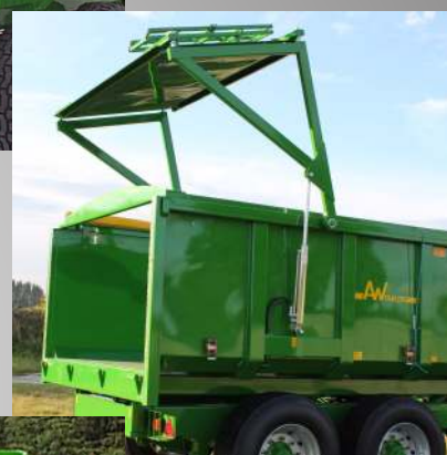
Contractor Hydraulic Tailboard
