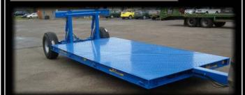
The standard Low Loader Trailer has a flat bed with a single axle at the rear which is hydraulically operated so that the bed can be lowered to the ground for easy loading and then raised for travelling. This trailer is designed to transport agricultural implements such as power harrows and drill combinations.
