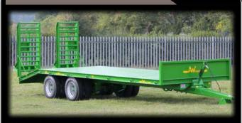
This has tandem axles under a flat bed with a beaver tail and fold down ramps at the rear for easy loading. It is designed to carry wheeled or tracked plant and equipment including diggers and excavators.
