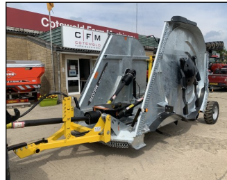
New Bednar MZ6000 mulcher/ripper, 6m working width, 3m transport width, 1000 PTO speed, galvanized body. £17,450
