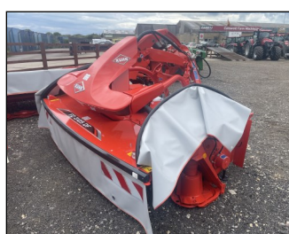
New Kuhn FC 3125 DF-FF front mower conditioner, 3.1m working width, hydraulic lift, steel tine conditioner. £POA
